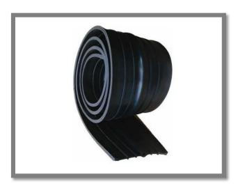
PVC Water Bar is a hydrophilic PVC waters stopper designed for waterproofing all types of concrete construction joints for civil engineering and building constructions. PVC Water Bar is capable of sealing heads of water up to 50 meters and is widely used to seal horizontal and vertical construction joints for poured in-situ concrete. It treated with a delay coating thus preventing it from premature expansion.
